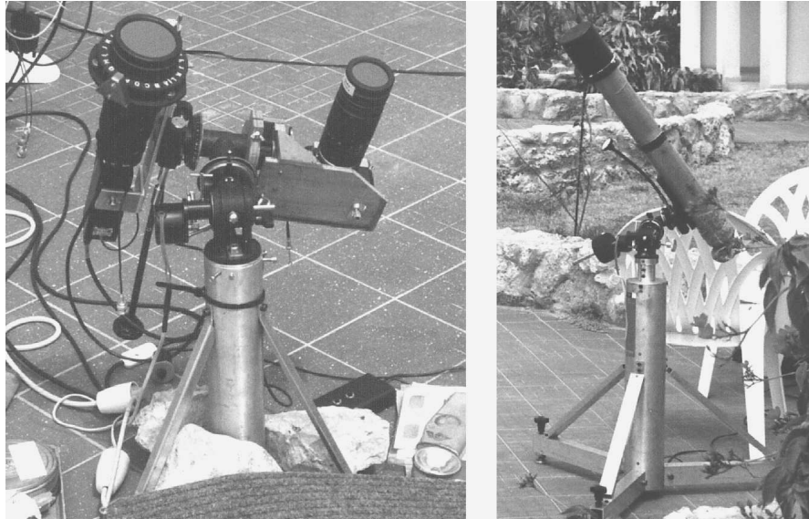
Figure 2. The two instruments used at the Curaçao observing station, February 1998. Left: the CCD imaging instrument showing the indexed circle of the polaroid filter. The SLR camera serves as a guiding scope as well as a counterweight and is also used to take some colour pictures of the eclipse after completion of the scientific program. Both camera's are equipped with 5-density neutral filters (calibration configuration), which are removed during totality. Right: the photographic instrument, a 1 meter focal length refractor, equipped at its prime focus with a polaroid filter with 6 indexed angular positions.
