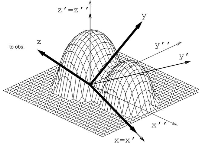
**Figure 1.** Definition of the ‘body frozen’ frame  $(x'', y'', z'')$  with the  $z''$  axis corresponding to the intrinsic rotation axis of the model and the ‘line of sight’ frame  $(x, y, z)$  with  $z$  pointing to the observer.
