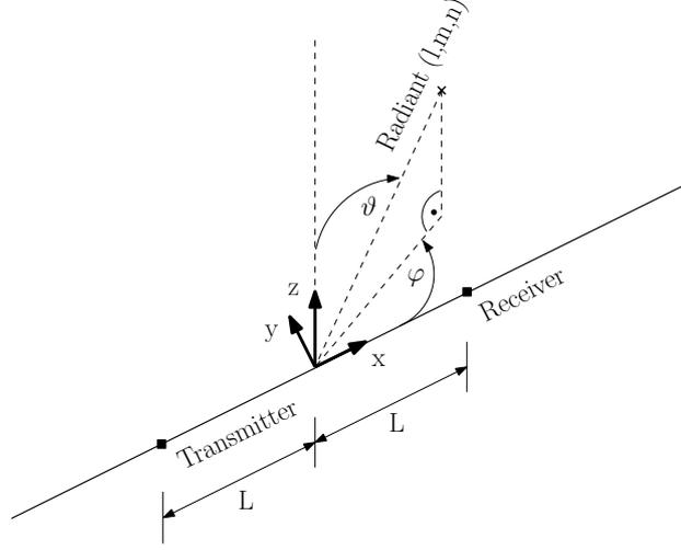
**Figure 2.** Coordinate system of the forward scatter setup.
