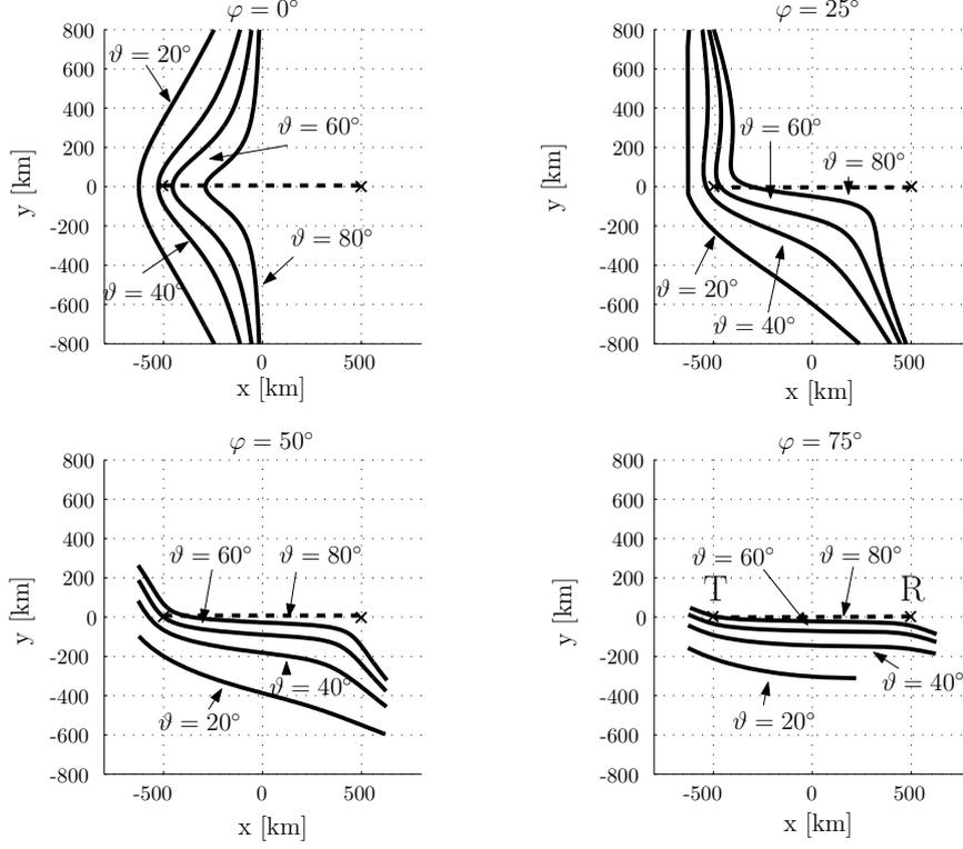
**Figure 3.** Examples of the curves of specular scattering points for various positions of radiants ( $\varphi, \vartheta$ ). The curves are calculated for T-R path distance of 1000 km and height  $h = 100$  km. The T-R baseline is depicted by a dashed thick line.
