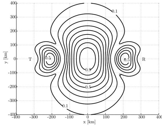
**Figure 4.** Combined theoretical gain factor of the transmitter and receiver antenna of the Bologna - Modra system (T-R path distance 612 km) at a 100 km height projected on the  $x, y$  plane.
