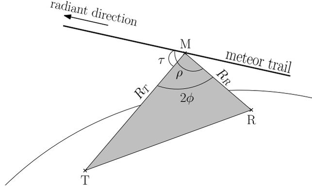
**Figure 1.** Geometry of the forward scatter system.  $R_T$  and  $R_R$  are distances from the reflection point  $M$  to the transmitter  $T$  and receiver  $R$ , respectively. The angle  $2\phi$  is a forward scatter angle and  $\tau$  and  $\rho$  are the angles between the axis of the meteor trail and directions to  $T$  and  $R$  in the point  $M$ , respectively.
