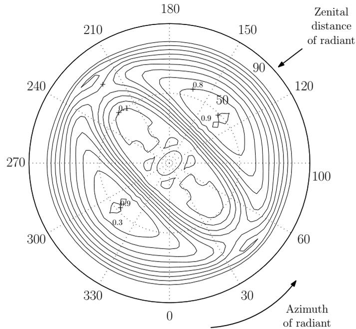
**Figure 5.** Observability function of the Bologna - Modra forward scatter system as a function of the azimuth and zenital distance of a radiant. The function is normalized to a maximum value of 1.
