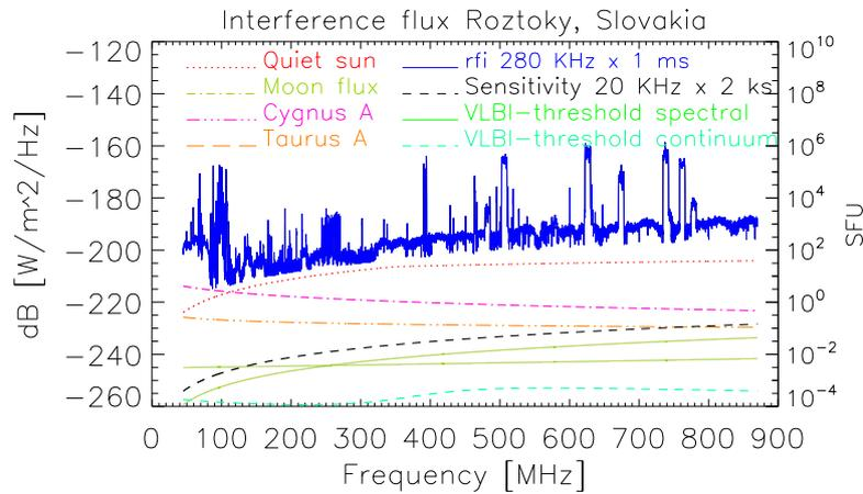
**Figure 13.** A spectral overview expressed in flux units for comparison with quiet Sun, Moon and other celestial radio sources. Also shown are current sensitivity and potential sensitivity with a long integration time of 2000 seconds. In addition, the plot shows the VLBI threshold level for spectral and continuum observations according to ITU-R RA.769. (ITU, 2002)
