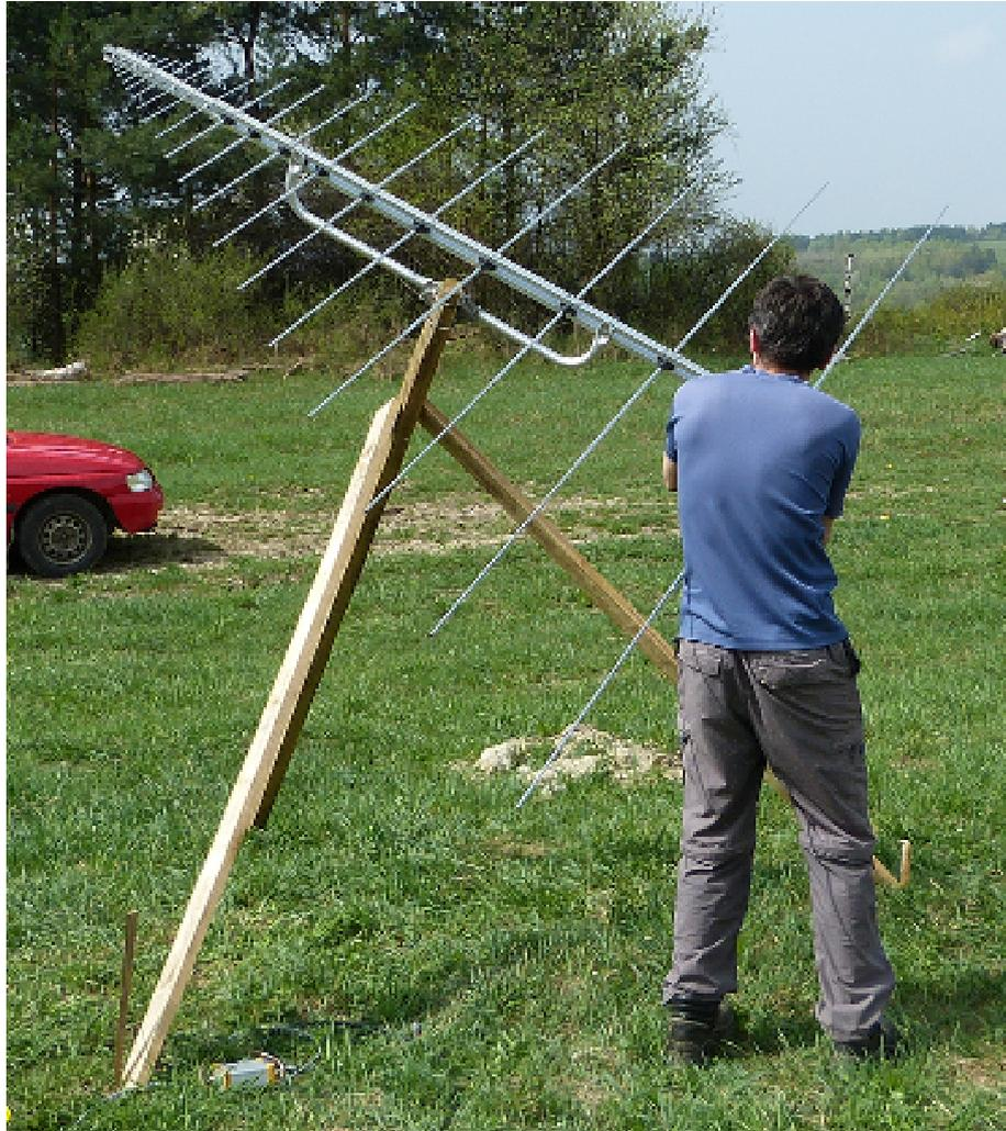
**Figure 1.** The logarithmic-periodic antenna CLP-5130-1 from CREATE at the Calisto observing station in Roztoky during its installation and configuration. The antenna, dedicated to observations of solar dynamic flares is mounted on a temporary wooden tripod positioned to the current position of the Sun.
