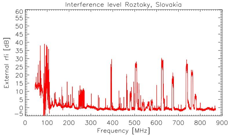
**Figure 2.** A spectral overview with 13'200 channels from a log-periodic broadband antenna measured at the Roztoky observing station. The spectra show some strong FM-transmitters around 100 MHz, TETRA at 400 MHz and DVB-T above 500 MHz. The negative dB in the FM range around 85 MHz indicates that the system is saturated. The plot also shows downlink transponder signals from military satellites near 250 MHz, indicating good sensitivity of the whole system.
