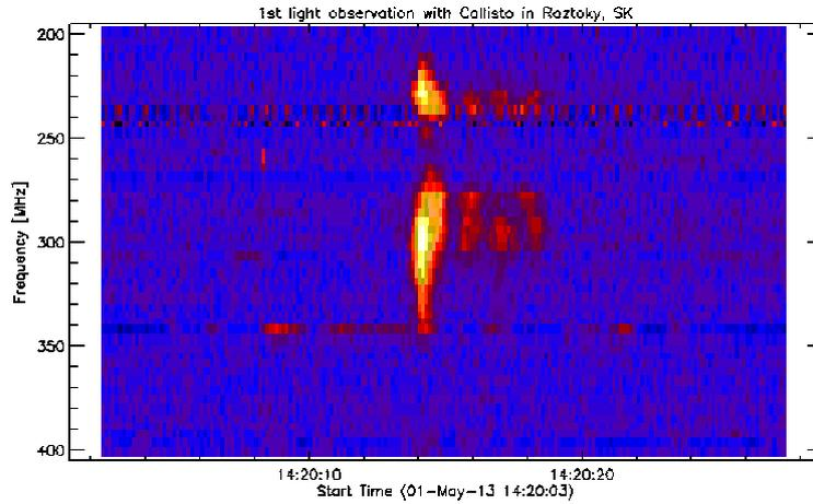
**Figure 12.** 1st light at Roztoky observed with the Callisto radio spectrometer showing a small type III burst (1st of May burst). Horizontal stripes are produced from local interference. A time resolution is of 250 ms and the spectrum is composed of 200 frequency channels. Each channel can be freely preprogrammed in the Callisto between 45 MHz and 870 MHz.
