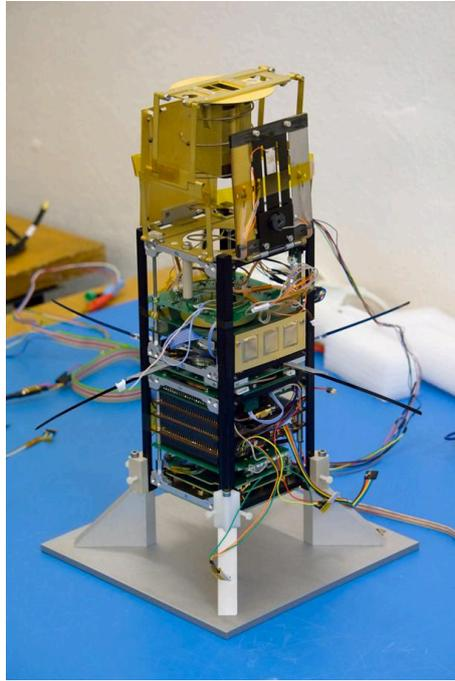
**Figure 3.** VZLUSAT1 2U cubesatellite with miniature X-ray telescope/monitor (in space extendable to 3U)
