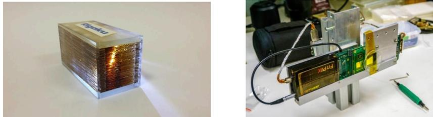
**Figure 1.** LE 1D optical module of the VZLUSAT1 miniature X-ray telescope (left) and the Widepix pixel detector (right). Widepix is pixel detector from the MEDIPIX family with 256 x 256, 55  $\mu$ m pixel size, 14 mm x 14 mm area
