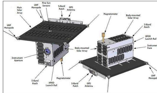
**Figure 4.** Small scientific satellite BRITE CZ with payload UV-BRITE and X-BRITE
