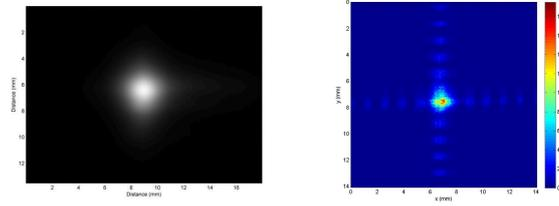
**Figure 2.** Image of point like source by 2D LE test module developed for NASA rocket experiment (Dániel et al., 2017) in optical light (left) and 8keV X-rays (right). The X-ray measurements were performed at the PenState X-ray test facility and the measured FWHM was 1.7 arcmin.
