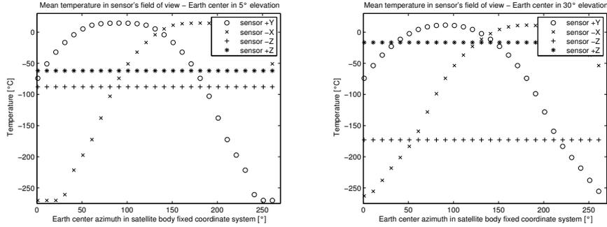
**Figure 3.** Theoretical temperature visible in TPS230 sensor's field of view dependencies on the actual Earth center position in the satellite body fixed coordinate system.
