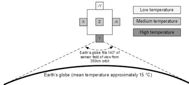
**Figure 1.** Placement of sensors for coarse attitude determination system.
