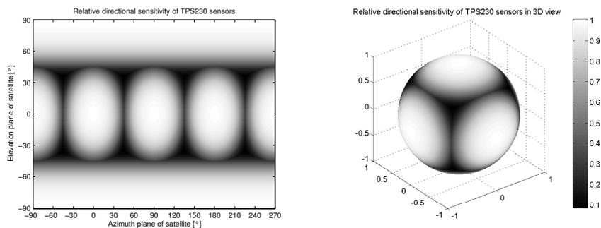
**Figure 2.** Omni-directional sensing system with six sensors, their placement and relative directional characteristics in satellite fixed body coordinate system.
