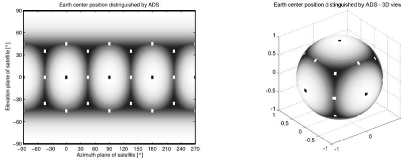
**Figure 4.** Earth center position distinguished by ADS - black marked positions by selection only the highest measured temperature, white marked positions added by selection and comparison of the three highest temperatures.
