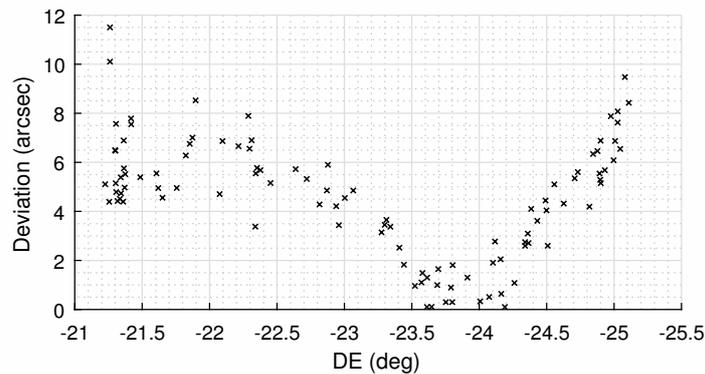
**Figure 3.** 3D plot of angular deviations from linear astrometric solution combined data RA and DE view from declination - deviation plane. Right ascension axis is oriented towards inwards.
