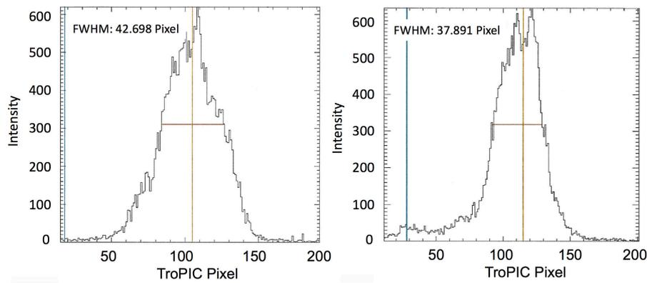
Figure 6.: The KB 2D X-ray optics – left FWHM of focus in vertical direction (3.2 mm), right FWHM of focus in horizontal direction (2.8 mm) at 1.49 keV.
