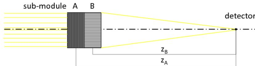
Figure 3.: Mounting configuration of the 2D-KB and LE optics during Panter tests.
