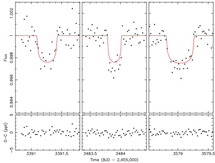
**Figure 4.:** Three primary transits of the circumbinary planet TOI-1338/EBLM J0608-59 and the photodynamical fit with its residuals (observed minus calculated). The variable transit duration, owing to a variable relative velocity between the star and planet, is a smoking-gun signature of a circumbinary planet. Figure reproduced from Kostov et al. (under review).
