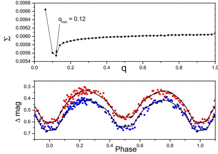
**Figure 1.** In the upper panel, the minimum mass ratio is determined to be  $q_{min} = 0.12$  with the  $q$ -search method. In the lower panel, the red and blue circles are  $R_C$  and  $I_C$  light curves, respectively. The black lines are theoretical light curves.
