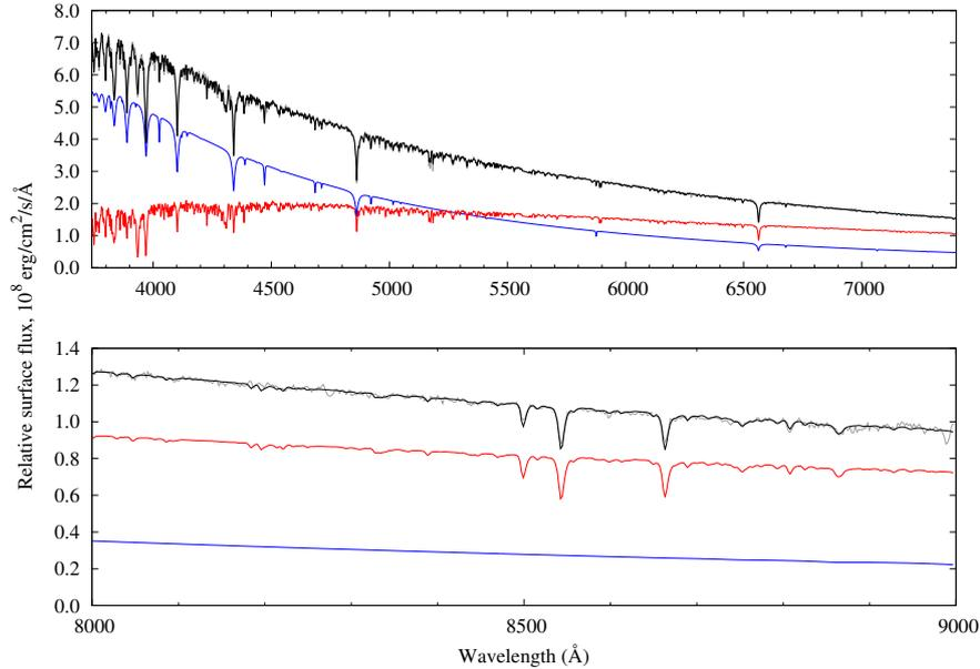
**Figure 1.** TLUSTY/XTGRID binary fit for the LAMOST DR1 composite spectrum of BD-75977 (grey line). The black model shows how the sum of an sdB (blue) and a G0V type model (red) fits the observation across the entire optical range. Further examples can be found at <https://astroserver.org/KW32YZ/>.
