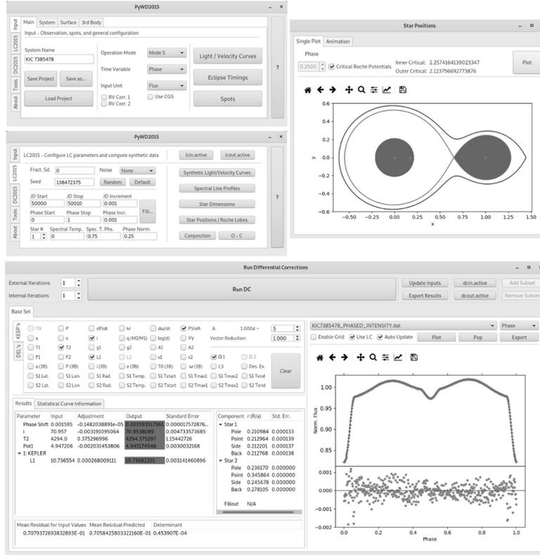
**Figure 1.** Representative windows of PyWD2015. Top left are the main and LC windows. The “Star Positions” window is at the top right. Below is the DC window.
