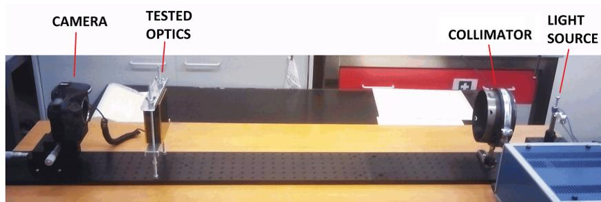
Figure 4. Experimental setup
